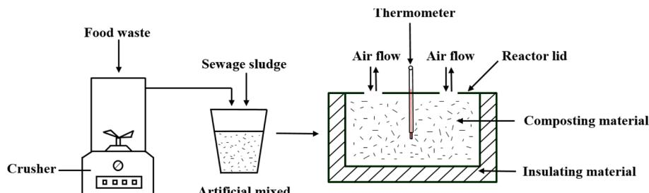
Fig. 1. Schematic diagram of aerobic composting.
