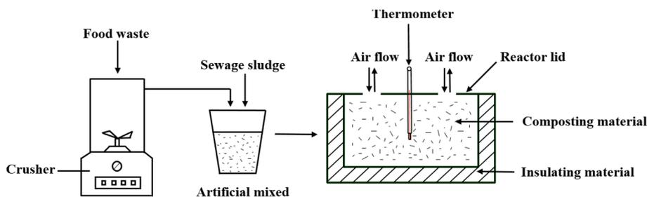
Fig. 1. Schematic diagram of aerobic composting.
